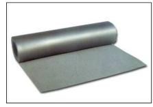
Plate made of closed cell expanded rubber AERSTOP N12 base EPDM e SBR, ASTM-D1056/77 RE 42. Used in industry for general purpose as seal for water, air and powder, lagging and soundproofing material. Good resistance to cold, ozone and ultraviolet rays, bad resistance to clorated solvents and to flame. Dimensions: mm 1000 x 2000, thickness mm 10.
