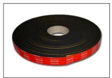
Section made of closed cell expanded rubber AERSTOP N12 base EPDM e SBR, ASTM-D1056/77 RE 42. Used in industry for general purpose as seal for water, air and powder, lagging and soundproofing material. Good resistance to cold, ozone and ultraviolet rays, bad resistance to clorated solvents and to flame. Packaged in cutable rolls with length m 50. Out of stock item.
