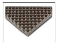
Adhesive soundproof panel made of open cell expanded polyurethan, base polyesther POLIESTIC PS 3000, with plane and rustication surfaces. Very good noise absorption coefficient, fire behavior UL-94HF-1. Packaged in cutable rolls with length m 25, height m 1, sold in square meters.
